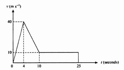
The diagram shows an approximate (t, v) graph for the motion of a parachutist falling vertically;  $v \text{ m s}^{-1}$  is the parachutist's downwards velocity at time t seconds after he jumps out of the plane. Use the information in the diagram
