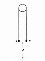
Particles A, of mass 5m, and B, of mass 3m, are attached to the ends of a light inextensible string. The string passes over a fixed peg, and the system is released from rest with both parts of the string taut and vertical, and each particle a distance d above a fixed horizontal plane (see diagram). Neglecting all resistances to motion,
